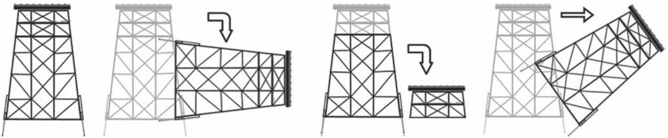
Fig. 3. Different decommissioning options: (a) leaving the rig unaltered in its current location; (b) toppling the entire structure in its current location; (c) partially dismantling the rig through “topping” – the removal of only the upper portion of the rig; (d) transport the rig to shore (Macreadie *et al.*, 2011).
