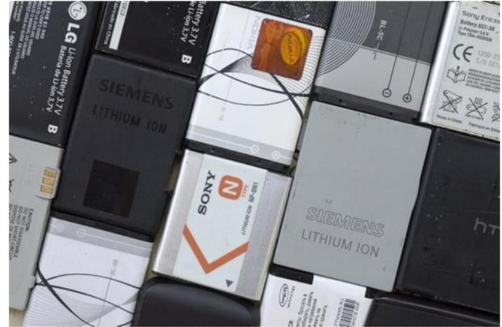
The diversity of cathode chemistries is a challenge because they may require different conditions for an efficient recycling process. Treating them simultaneously **increase the required resources** (e.g. energy and time consumed by a sorting mechanism) or may have a **negative impact on the quality** of the outputs.
